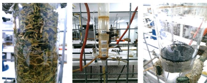
(Fig. 1. The culture media before adapting stage) (a) hemp; (b) biological sludge; (c) chemosorb
